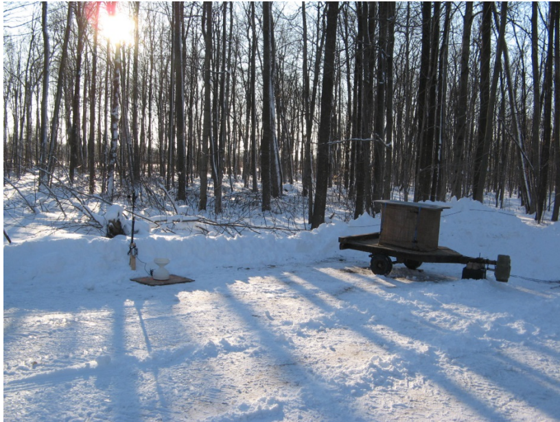
Figure 1 – Noise measurement location at the Weaver residence near Arthur, ON. 723 m away from the nearest IWT. Nearby: ONSET Wind Speed/Direction Smart Sensor model S-WCA-M003 with Onset HOBO Micro Station logger model E348-H21-002. Also, a tipping bucket rain gauge is co-located with the wind sensors. Microphone locations are situated in sheltered areas. Location: N4847853 E534398
