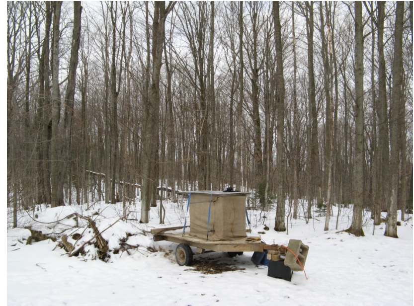
Figure 2 - Background noise location & setup: in a small clearing east of Eugenia Lake, Grey Highlands, ON. This site was chosen to be closely comparable to the Weaver location near Arthur. The microphone is located in a burlap wrapped wire crate on a trailer. Location: N4909221 E542872
