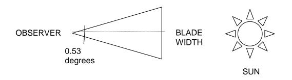
In the equation the 0.5 comes from the use of half the blade width to determine the straight line distance (the line splitting the triangle in half). The "tan 0.053 degrees" comes from using half the angle when 20% of the sun's disk is covered, or 0.5 times 0.2 (or 20%) times 0.53 degrees. For this 20% blockage of the sun's disk, an elevation of 0.8 degrees, and an estimated average blade width of 5 feet, the distance from observer to the tower's base would be about 2700 feet.
